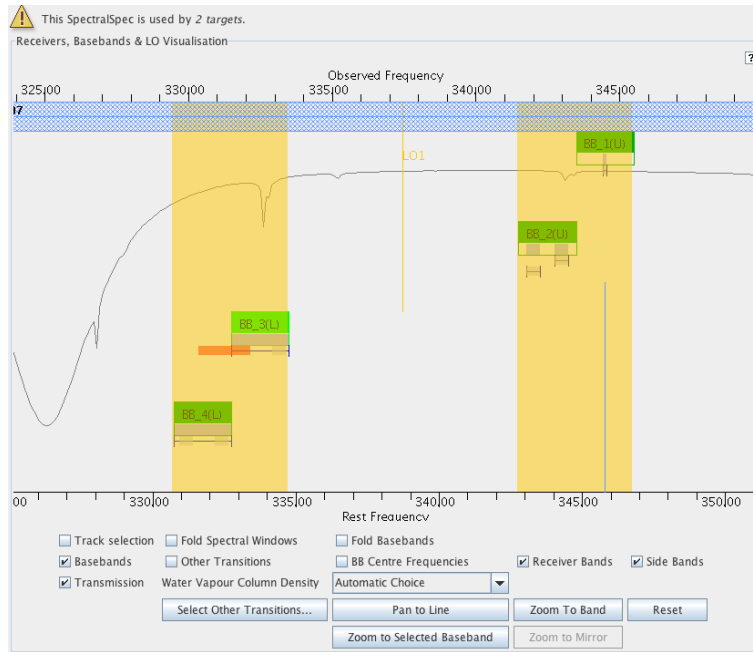
Figure 9.2: The graphical representation of the frequency information in a Scheduling Block. This is a zoomed view and hence the spectral windows and their spectral averaging regions can be seen. The basebands are shown as the green blocks and within these can be seen the spectral windows (horizontal bars). Below the basebands are the spectral averaging regions (also horizontal bars). Note that there are two spectral windows in Baseband 2, each with a single spectral averaging region. Baseband 3 contains a spectral averaging region which extends out of the spectral window and has thus been coloured orange to signify a problem.
